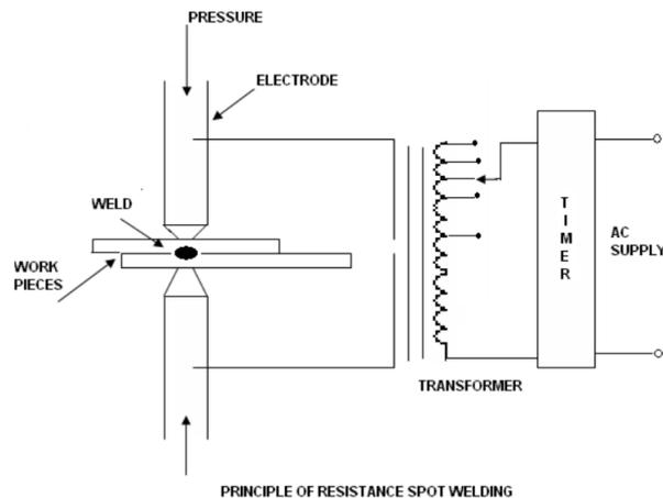
In resistance welding (RW) a low voltage (typically IV) and very high current (typically 15,000 A) is passed through the joint for a very short time (typically 0.25 s). This high amperage heats the joint, due to the contact resistance of the joint and melts it. The pressure on the joint is continuously maintained and the metal fuses together under this pressure. The heat generated in resistance welding can be expressed as
