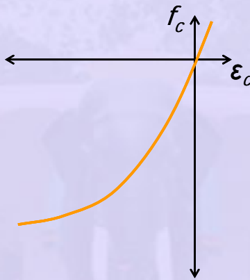
Figure 3-1.3 Stress versus strain for concrete
