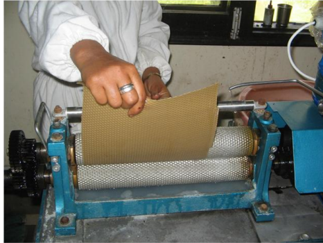
Figure 6.5 Comb Foundation Mill
